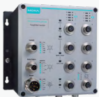
TN-5500A Series EN 50155 M12 Managed PoE Switches
